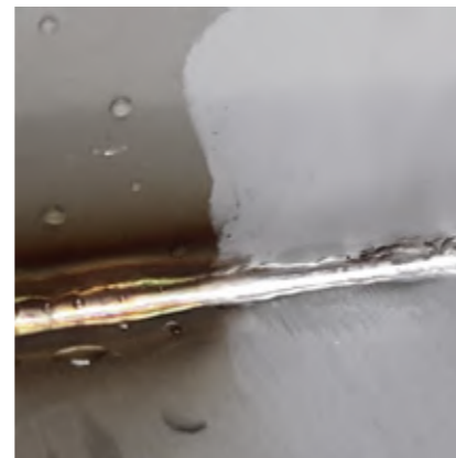
Before the treatment | After the treatment Cleaning of weld seams
